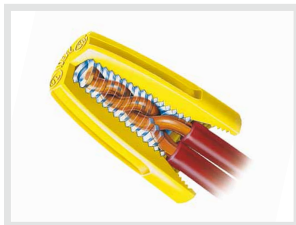
Wire-nut wire connector cross section
